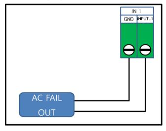
2 stated input ports to monitor controller box status of AC FAIL, LOW BATTERY, TAMPER ALARM and more NO/NC option
