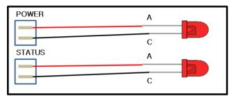
Output port for controller monitoring LED on the outside of controller box. POWER / BOARD STATUS / ETH\_TXD / ETH\_RXD / ETH\_STATUS Output voltage/current: 5V / 20mA (MAX)
