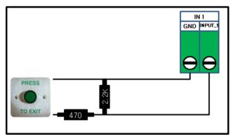
Inputs for sensors of exit buttons, door contacts, PIR and others
